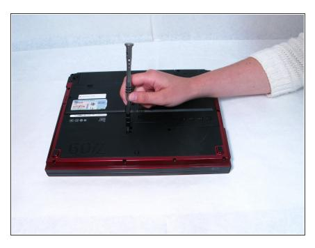
Remove all visible screws from the bottom of the computer.
