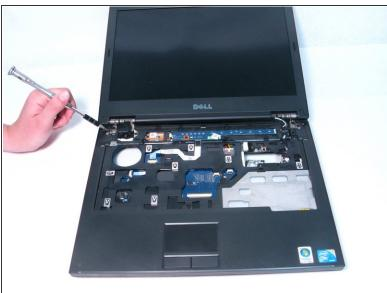
Undo the screws holding the screen to the computer base.
