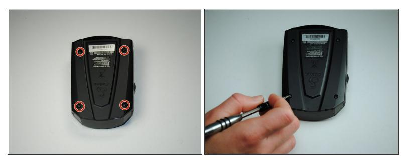
• Remove the four 9.5 mm Phillips #0 screws from the back of the device.
