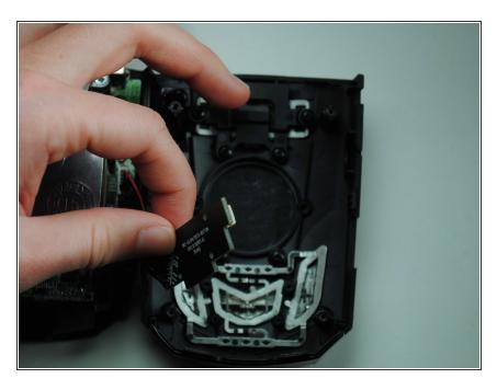
• Lift buttonboard to expose silver button plate.
