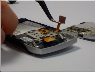
Use tweezers to disconnect the copper ribbon from the inside of the back panel.
