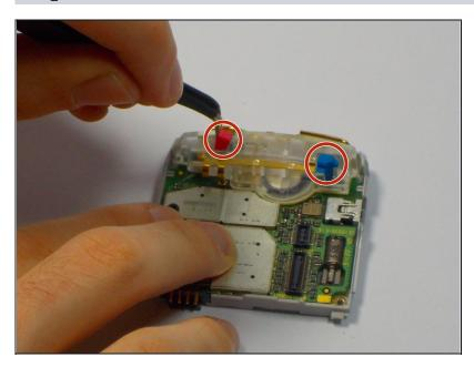
Use tweezers to remove the tiny red and blue rubber covers located on the top of the antenna.
