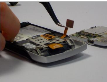
• Use <u>tweezers</u> to disconnect the copper ribbon from the inside of the back panel.
