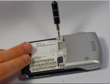
Remove the two screws from the back panel with a T6 screwdriver.
