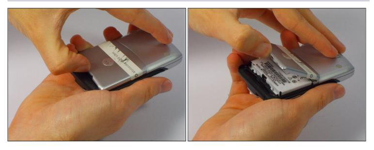
• Press the release button located on the upper edge of the battery cover. At the same time, lift the battery cover away from the phone.
