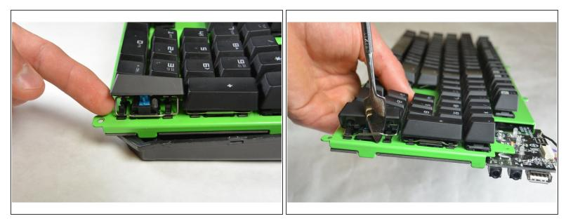
• For larger keys, such as the space bar or shift keys, the axel underneath needs to be released by gently pulling it out and away from the center of the keyboard with the metal spudger.
