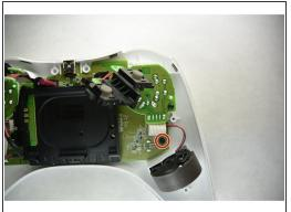
Now that the joysticks are removed, locate the screws on the left and right side of the controller (highlighted in the photos) and use the J0 bit to remove these 4 mm screws. This will allow you to pull out the controller board
