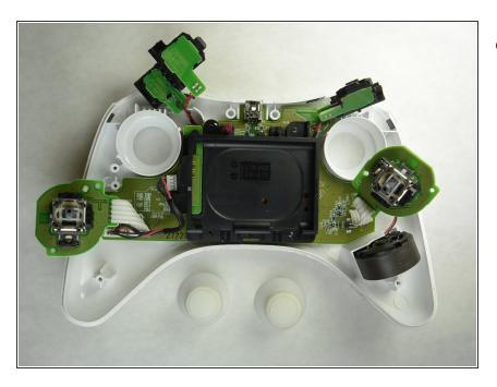
Carefully pull the rubber thumbsticks off of the electronic bearings to remove the joysticks.
