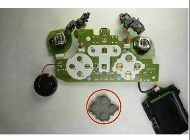
Remove the rubber covers (circled in the photo) from the ABXY sensors from the control board that was removed from the housing.
