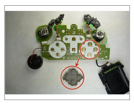
Wipe down the rubber cover pad completely with rubbing alcohol and a q-tip. Use compressed air to clean off the contact sensors (highlighted by the red circle). To reassemble your device, carefully follow these instructions in reverse order.
