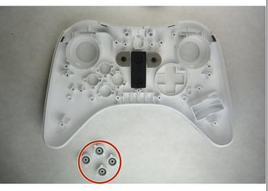
Once these two screws have been removed, you may go ahead and remove the board from the
