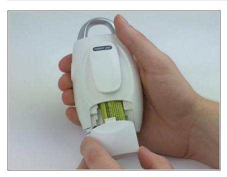
Remove the battery cover by sliding it down.
