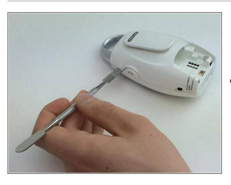
Using a plastic opening tool, pry apart the front part of the device from the back. There are many
