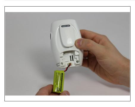
Firmly grasp the battery and pull to disconnect the battery from its connector.
