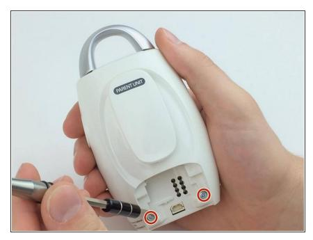
Using a Phillips #00 screwdriver, unscrew the two 5.0 mm screws located at the bottom of the monitor inside of the device.
