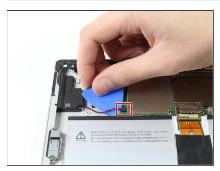
Use the pick to gently lift on the red and black wire in order to dislodge the connection between the speaker wire and the motherboard.
