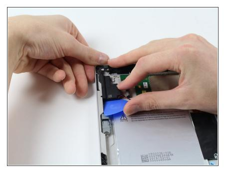
Use a pick to get under the speaker part and undo the adhesive that keeps it attached to the back casing.
