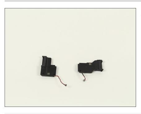
Simply replace the old speakers by snapping the new speakers into place and connecting the red and black wire to the motherboard.
