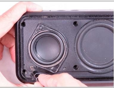
Remove the one 7-mm Phillips head screw located on the lower left of the front of the speaker with the PH1-bit screwdriver.
