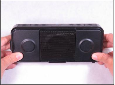
After all screws are removed, turn the speaker over to the back of the speaker.
