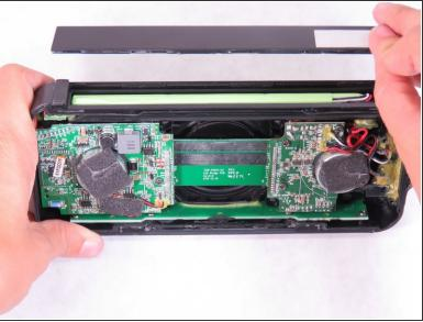
• Then remove the bottom narrow strip of plastic to uncover the battery.
