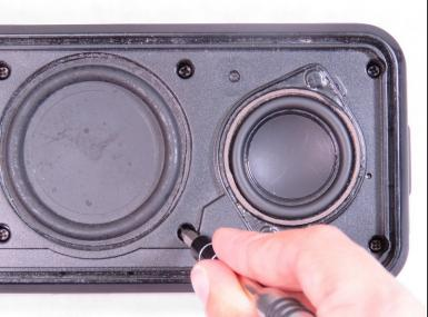
Use the PH1-bit screwdriver to remove the eight 11-mm Phillips head screws that are located behind the faceplate.
