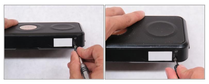
Use the T09-bit screwdriver to remove the two 8-mm torx screws on the bottom strip of the speaker.
