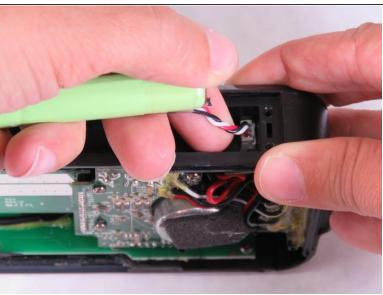
Follow the red, black, and white wires attached to the green battery sleeve down to the white small plug.
