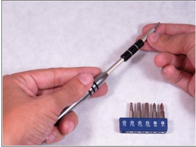
• Obtain the screwdriver and the T09 (Torx) bit from the iFixit toolkit and assemble them together.
