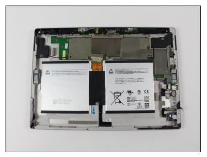
Now that you've gotten the casing off of the Surface 3, you can start removing the battery pack.
