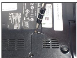
Remove the four 4.76 mm Philips screws on the back of the laptop using the Phillips J0 Screwdriver.
