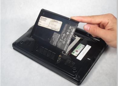
Use a plastic opening tool to remove the back cover.
