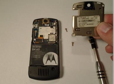
• Once you have removed all of the screws, lift the transceiver PC board shield up to remove it.
