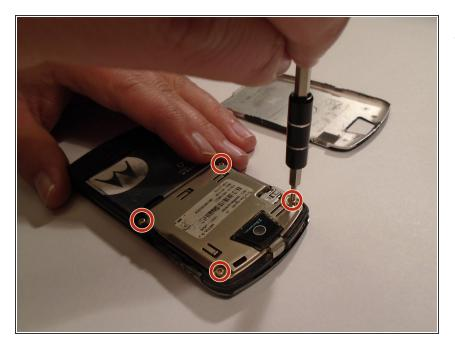
Remove the four housing screws
