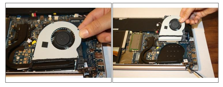
• Gently lift and slide the cooling fan out.
