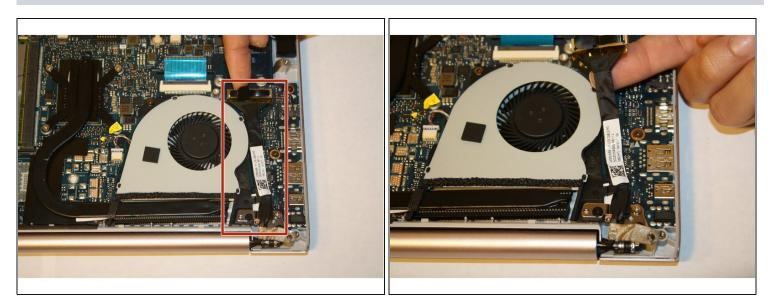
• Pull on the black flap to lift the LVDS cable next to the cooling fan.
