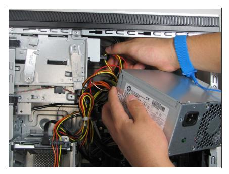
Unplug the power cable going to the CD drive by pulling straight.
