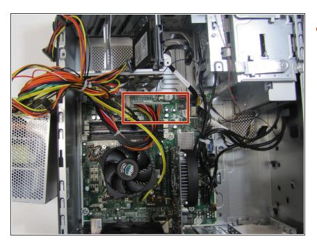
Unplug the power cable going to the mother board by pulling straight up.
