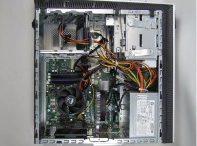
Remove the side panel by sliding it towards the back of the desktop and pulling up on it as shown.
