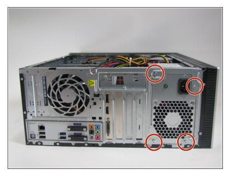
Remove the four 5mm screws holding the power supply in place with a T15 Torx screwdriver.
