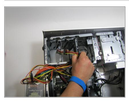
Unplug the SATA interface power cable going to the hard drive by pulling straight up.
