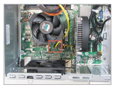
Unplug the power cable going to the fan by pulling straight up.
