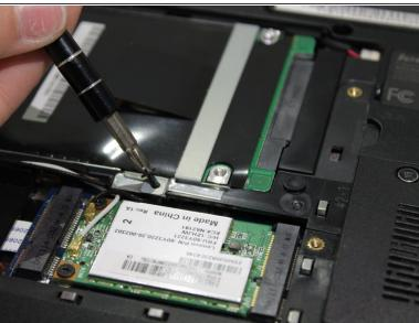
• Remove the 40 mm screw using a Phillips J0 head screwdriver.
