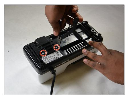
Remove the two hex-cap screws on the bottom using a pair of pliers.
