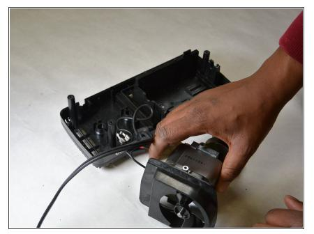
Remove the motor and shaft assembly from the bottom of the case housing.
