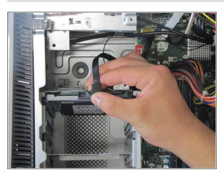
Finish disconnecting the hard drive by unplugging the black SATA interface cable by pulling up.
