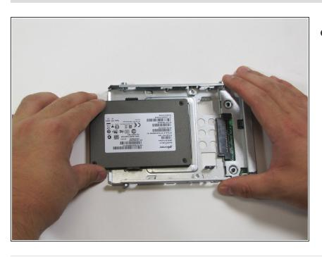
Finally, slide the SSD out of the casing.
