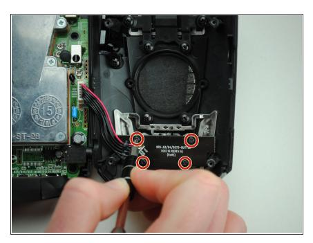
Remove the four 4.8 mm Phillips #00 screws from the buttonboard.
