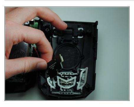
Lift buttonboard to expose silver button plate.
