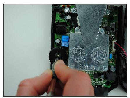
Remove the one 4.8 mm Phillips #00 screw from the center of the audio dial.
