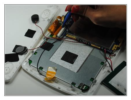
Use a plastic opening tool to release the three ribbon cables attached to the motherboard.
