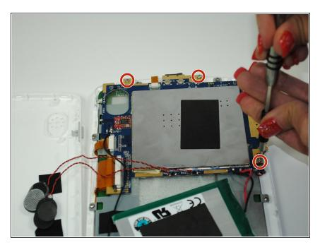
Use a screwdriver to remove the three 7.0 mm Philips #00 screws and unscrew the motherboard.
