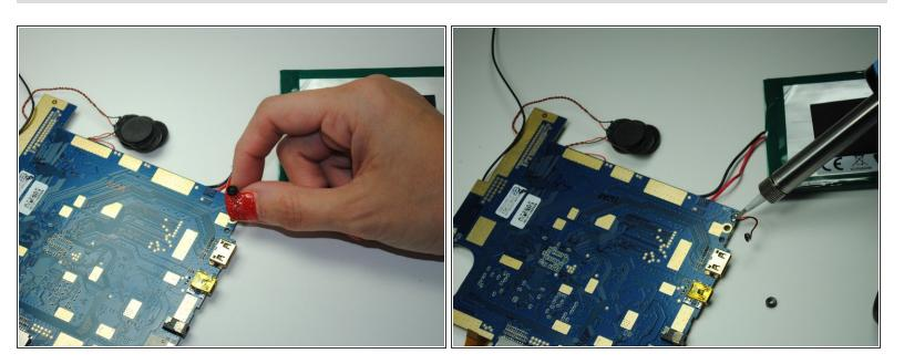
• Lift up the motherboard and use a soldering station to remove the microphone from its wires.
