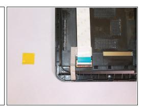
Use the wide nosed tweezers to remove the yellow tape that secures the bottom end of the ribbon cable. Gently lift the edge of the tape.
