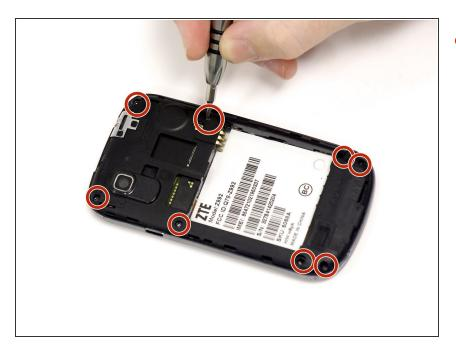
Using your J00 screwdriver, unscrew each of the 8 Philips head 1.19mm screws from the black plate of the device.
