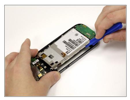
Using an opening tool, lift and remove the silver metal plate off the back of the device (use some force here).
