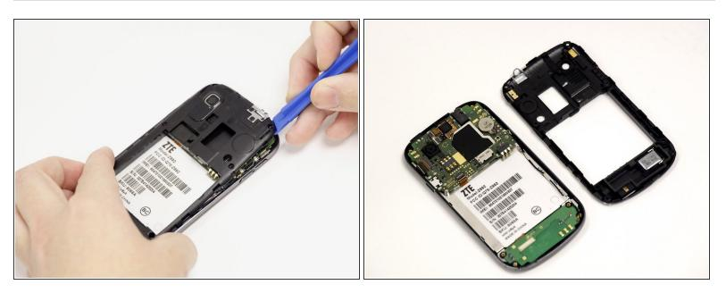
Using a spudger or plastic opening tool, pull up from underneath the back plate and pop off the piece.
