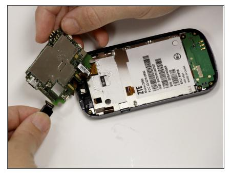
• Lift and set aside the motherboard from lying on top of the silver plate (this may require some force because it is held on by adhesive).
