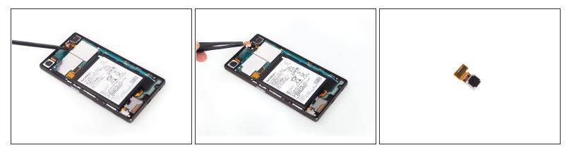
• Release front camera connector and remove front camera.
