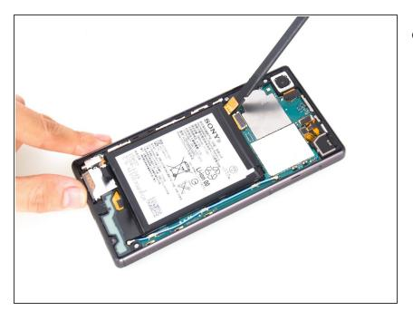
Release battery connector in order to prevent short circuit.
