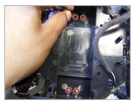
Remove the four 13 mm Phillips #1 screws.
