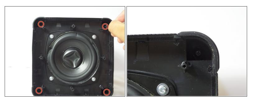
• Remove the four 13 mm Phillips #1 screws.
