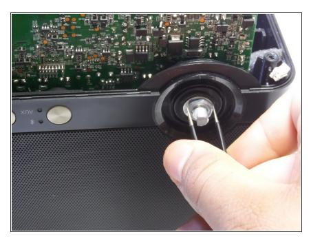
Using tweezers, turn the nut counter-clockwise and remove the nut.
