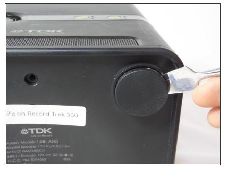
• Remove the four rubber feet of the device using a metal spudger.
