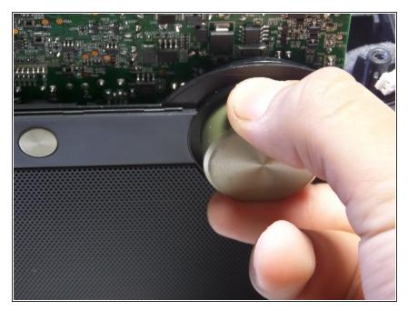
Remove the volume control knob, which is located at the front of the speaker, by pulling it towards you.
