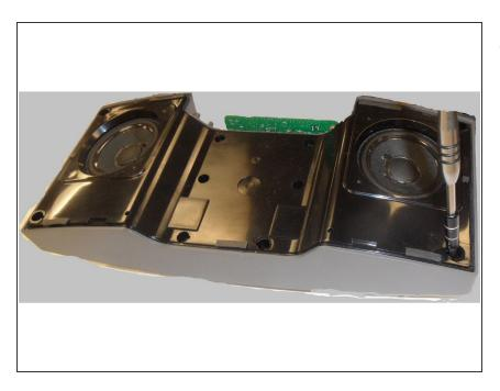
Use a #2 screwdriver to remove the six 8.5 mm length screws from the speaker cover.
