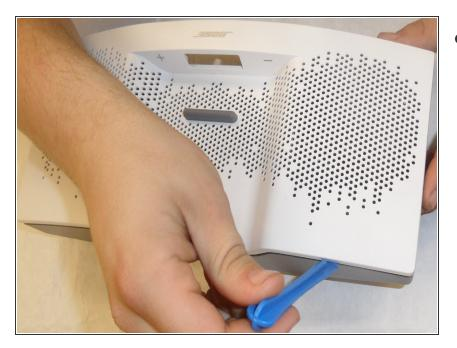
Next, use a plastic opening tool to slide under the edge of the front cover. Start edge located at the top of the left or right speaker and work your way around the speaker. Remove the front cover.
