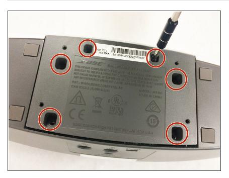
Remove six 10 mm length screws from the bottom panel of the SoundDock.XT using a #1 Phillips screwdriver.
