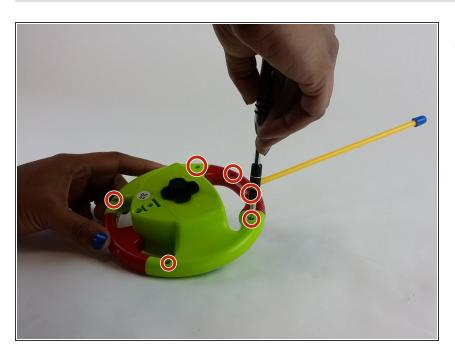
Flip the remote control and unscrew all the six 6.5 mm screws with the Phillips #00 screwdriver.
