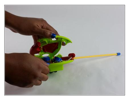
Pull the device apart to find the connection between the antenna and the white wire.
