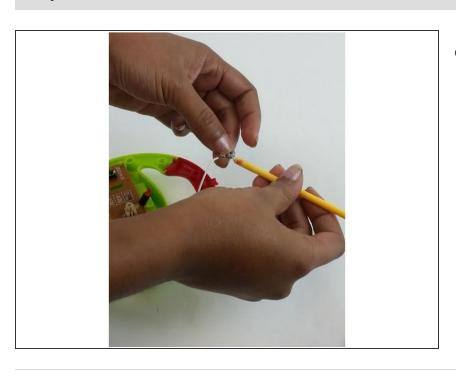
Replace the old antenna with a new one. Attach the new antenna to the white wire and screw it in place.
