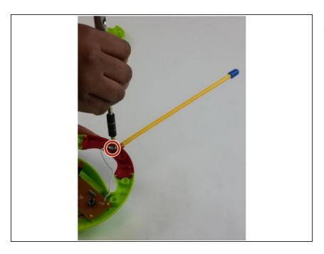
Unscrew the 4.5 mm screw that attaches the antenna in place.
