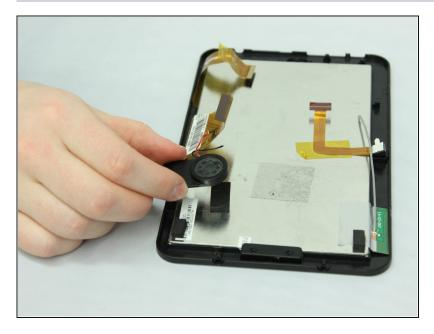
• Using thumb and forefinger, remove the speaker unit from the device
