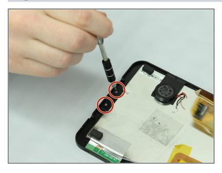
Using a J000 Philips head screwdriver, remove the two 5mm screws that hold the display unit down at the bottom of the device, turning the screws counterclockwise.
