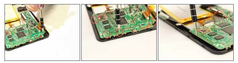
• Use the PH000 screwdriver remove the four 5 mm screws along the bottom edge of the motherboard, turning them counterclockwise.
