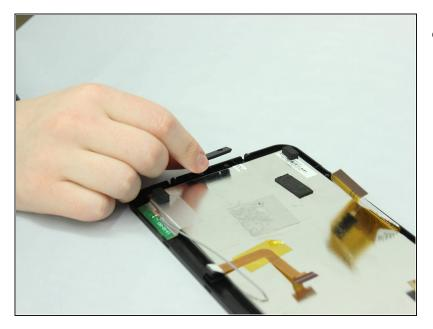
Lift the small black display protector that was between the screws and the display unit using your forefinger and thumb.
