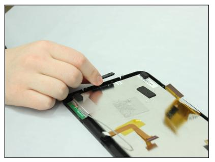
Lift the small black display protector that was between the screws and the display unit using your forefinger and thumb.
