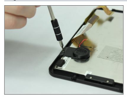
Remove the 5mm screw that holds the speaker unit on to the display unit using a J000 screwdriver, turning the screws counterclockwise.
