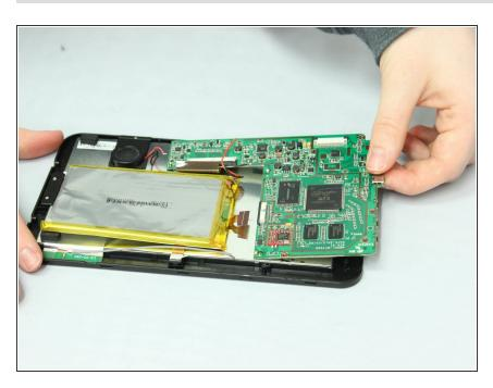
Using your index finger and thumb, lift the motherboard out of the device.
