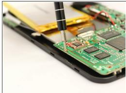
Use the PH000 screwdriver remove the four 5 mm screws along the bottom edge of the motherboard, turning them counterclockwise.
