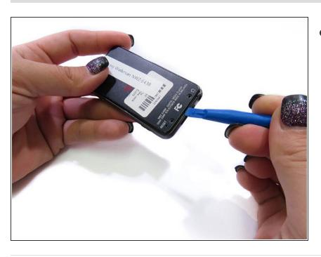
Use a small prying tool to carefully pry open the back of the device.
