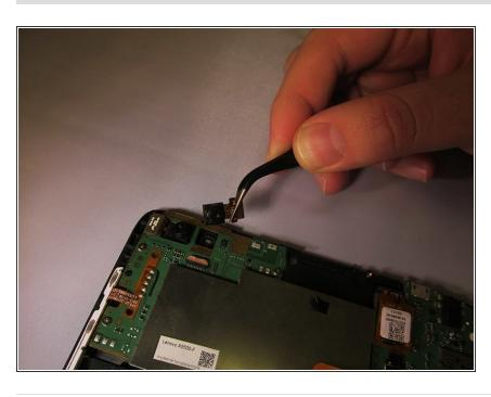
Using tweezers to grasp the camera connector, lift the camera out of its socket.
