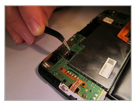
Using tweezers, peel off the antistatic sticker from the camera connection port.
