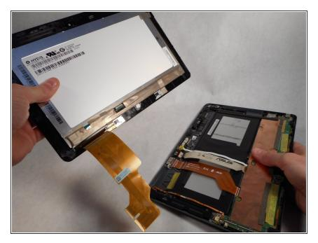
• Lift the screen upwards to remove.
