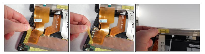
Remove the yellow tape covering the end of the cables.
