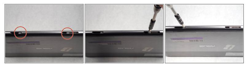
• Rotate the device 180°, and remove the two 1.59 mm screws at the bottom of the device.
