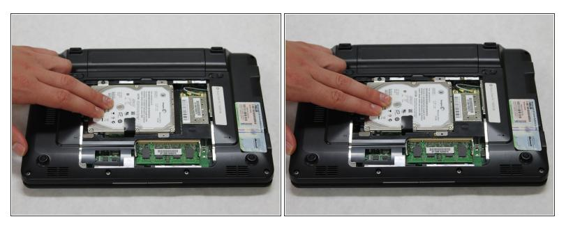
• To remove the hard drive, slide it to the right.
