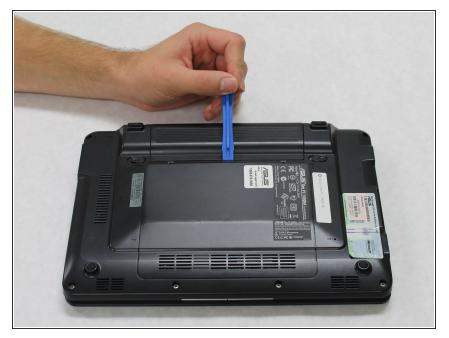
Place the blue plastic 1/4" opening tool into the small indention and gently pry the back panel off.
