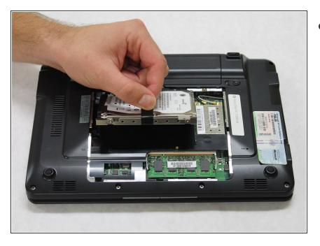
• Grab the black tab and lift up to remove the hard drive from the computer.
