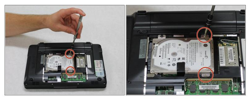
• Use the same, #00 Phillips Head screw driver to remove two 1/8" screws.
