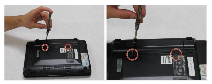
Use a #00 Phillips Head screw driver to remove the two 1/4" screws that hold the back panel in place.
