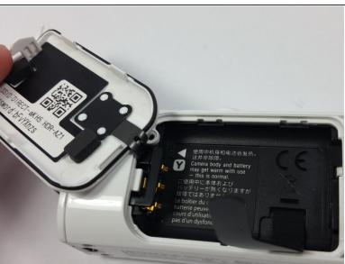
Remove the circled 4 millimeter black screw adjacent to where the door is attached.
