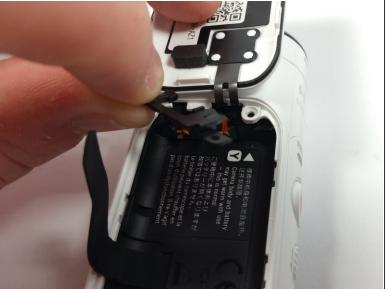
• Grab the small black bracket holding the ribbon on which the door is attached and pull it out.
