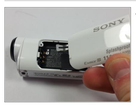
Pull the door straight back so the attaching ribbon is pulled taught and the door will come right off.
