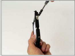
Remove four 3.5 mm PH#0 screws on the sides of the hard drive.
