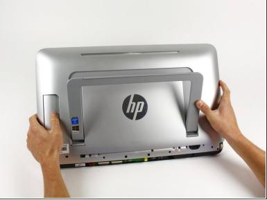
Release the stand by pressing the large button on the left so that it is easier to take the back case
