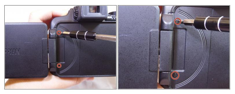
Use a Phillips screwdriver to unscrew the two 5.556 mm screws under the LCD screen.
