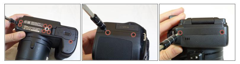
Use a Phillips screwdriver and remove the eleven 5.556 mm screws around the outside frame of the camera.
