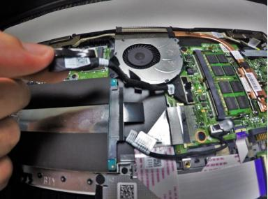
• Remove the cord that runs from system board to the I/O board.
