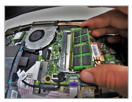
Pull the Memory Module from its slot by grasping each side with thumb and middle or index finger to pull from the rest of the device.
