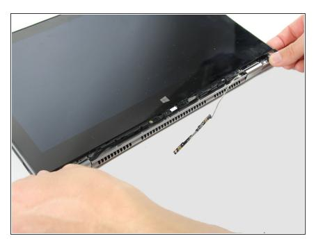
Slide the screen up away from the hinges and lift from the backplate.
