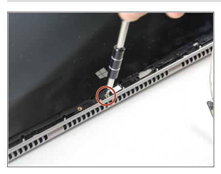
Remove the last 1/8" screw near the middle of the screen using a Phillips #00 screwdriver.
