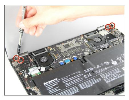
Remove the four 3/16" screws from the top of the laptop near the hinges using a Phillips #00 screwdriver.
