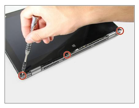
Remove the three 1/8" screws using a Phillips #00 screwdriver.
