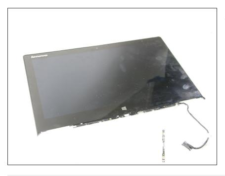
Carefully remove the hinges and remove the screen.
