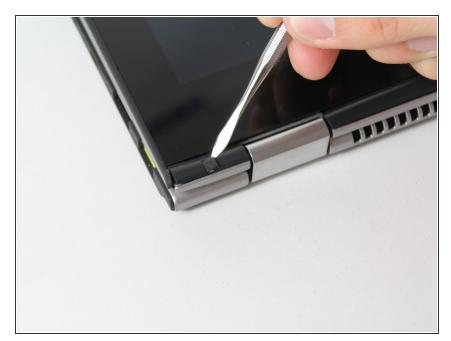
Open the laptop and remove the two screw covers on either side of the computer near the hinges using either the tip of a flathead screwdriver or a spudger.
