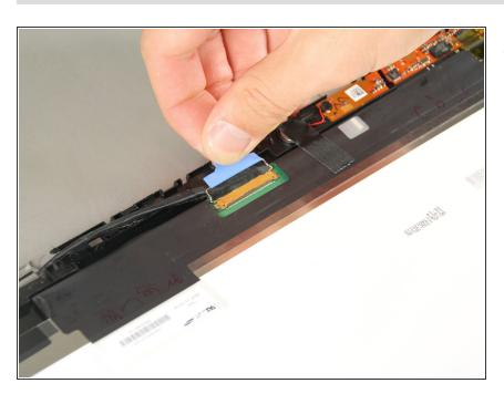
Fold the screen over and disconnect the LCD screen cable by lifting up the blue tab and pulling.
