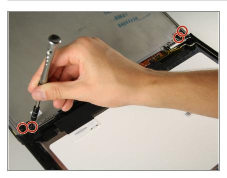
Remove the four 1/8" screws using a Phillips #00 screwdriver from the hinge on either side of the laptop.
