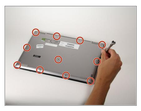
Using a Torx T5 screwdriver, remove the eleven 1/4" screws from the back of the laptop.
