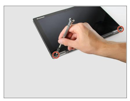
Remove the revealed two 3/16" screws using a Phillips #00 screwdriver.
