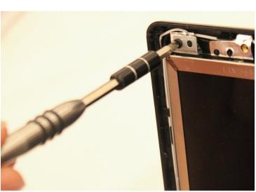
• Use a Philips #1 screwdriver to remove the top left and right two 7 mm Phillips #1 screws by turning the screws counter clockwise.
