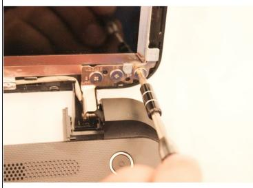
• Use Phillips #0 screwdriver to remove the six, 2.5 mm screws on the bottom left and right, by rotating the screwdriver counterclockwise.
