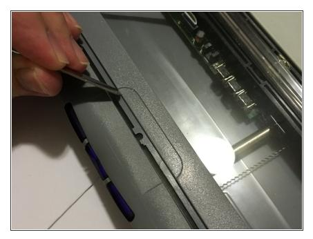
Use your hands or a metal spudger tool to push the plastic bar at the bottom of the glass scanner bed forward until you can't push it any farther.
