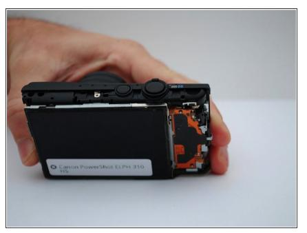
• The back side of the camera should pop off or be removed by hand.
