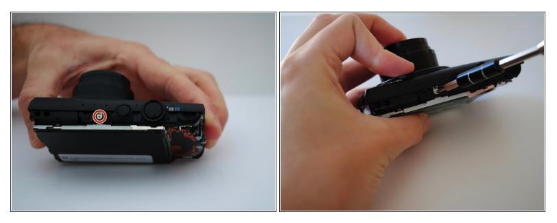
• Unscrew the one 3 mm Phillips head screw on the top of the camera.
