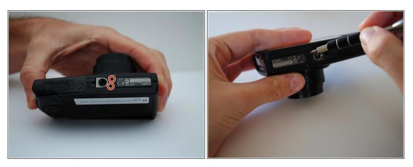
• Unscrew the two 4 mm Phillips head screws from the bottom side of the camera.
