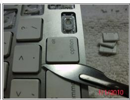
Here we can see the different types of key mounting and scissor mountings
