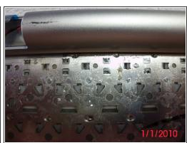
There are ten 2 mm screws located on the back of the board.
