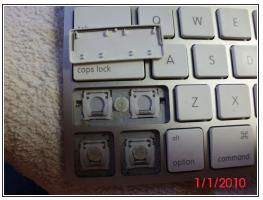
Keys can be easily removed by using a scalpel or fingernail under the left side and lifted.
