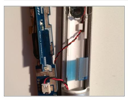
Using the tip of a spudger, flip up the keyboard ribbon cable retaining flap.
