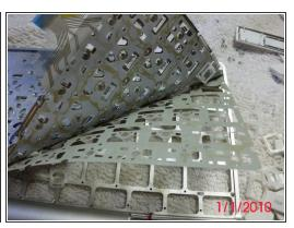
• The layers are pulled apart. Frame, plastic separator layer, printed circuit layer
