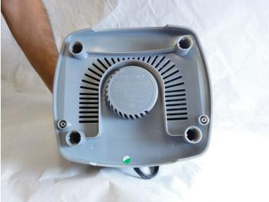
• Use a spudger to remove the 4 rubber base pads located at the corners of the device.
