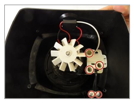
Remove the screws indicated with a screw driver.
