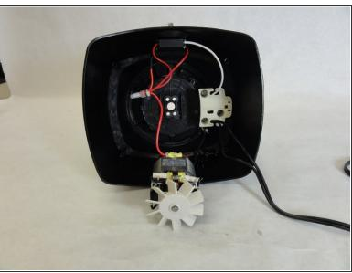
Remove the remaining screws to unhinge the motor located at the center of the device using a screw driver.
