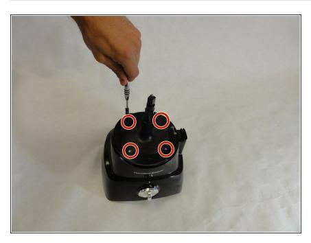
Remove the 4 screws located under the plastic caps with a screw driver.
