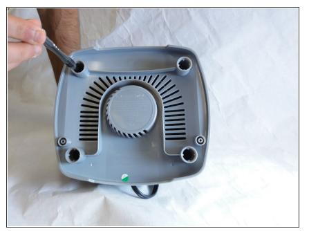
Unscrew all 4 screws that are located beneath the pads with a screwdriver and remove the plastic grey base.
