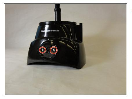
Remove the two screws behind the knob with a screwdriver.
