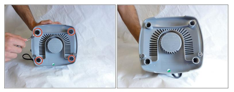
• Use a spudger to remove the 4 rubber base pads located at the corners of the device.
