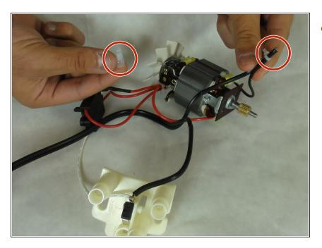
Remove to electrical cap to the positive terminal(black terminal), and undo the wiring.
