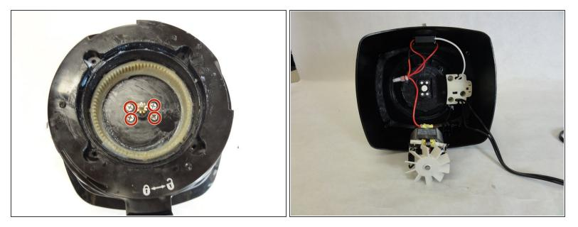
Remove the remaining screws to unhinge the motor located at the center of the device using a screw driver.
