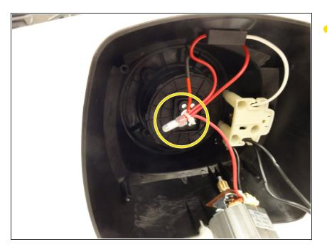
Remove the electrical cap to the negative end(red wire), and undo the wiring. Once this is complete reconstruct the wiring with the new motor.
