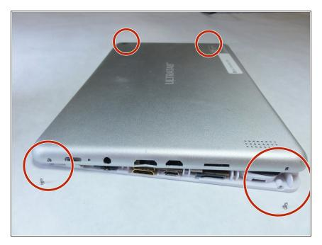
Remove the 4 exterior screws using a <u>Phillips #000 Screwdriver</u>.
