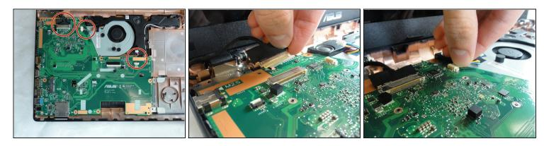
Disconnect the three cables attached to the motherboard.
