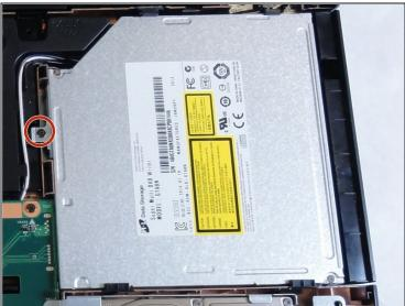
• Remove the single screw that is holding the drive in place using the Phillips #1 Screwdriver.
