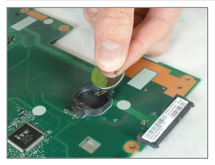
Lift the battery out of the housing.
