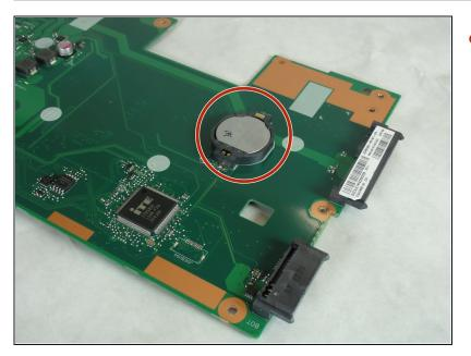
Locate the CMOS battery on the reverse side of the motherboard.
