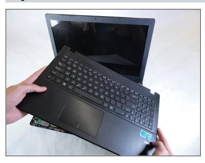
Remove the fully disconnected keyboard module from the laptop.
