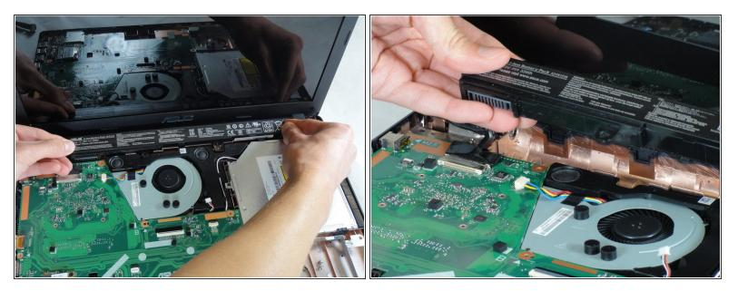
• Lift the battery out and remove it:
