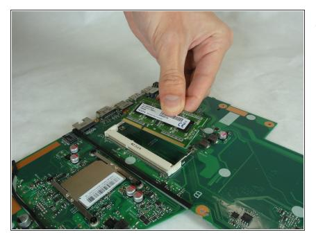
• Lift the RAM module out of its place.
