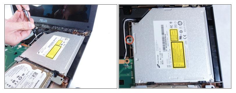
• Remove the single screw that is holding the drive in place using the Phillips #1 Screwdriver.
