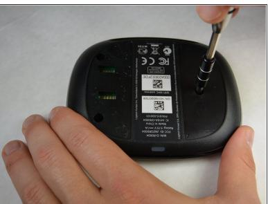
Using the PH00 bit, remove the four 6mm Phillips screws
