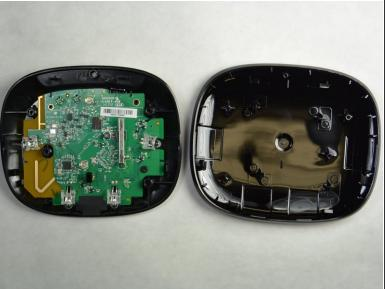
Use the plastic opening tool to pry open and separate the pieces of plastic from each other.
