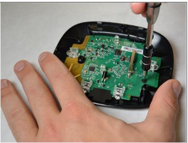
Using the PH00 bit, remove the three 4mm Phillips screws.
