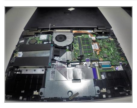
Lay the screen flat on a smooth flat surface to release the hinges.
