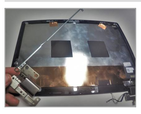
Grasp the hinge from the edge as shown and separate the hinge from the display. To reassemble your device, follow these instructions in reverse order.
